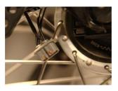
Reassemble the black cap and put the plug back on the dynamo.
