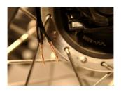
Thread the two twisted wires back into the gray plug and bend the copper wires according to the following picture.
