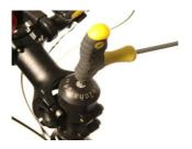
Prior to the final tightening of the screw, rotate the Cycle2Charge to have the USB outlet in the preferred direction.
